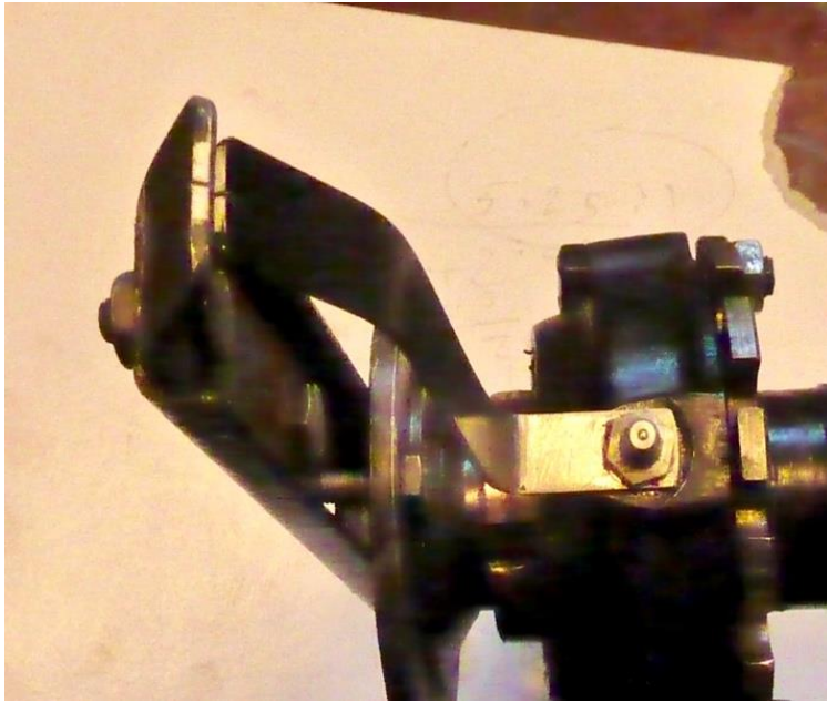
Index marks used to check 1/16" of backlash at 7" radius
